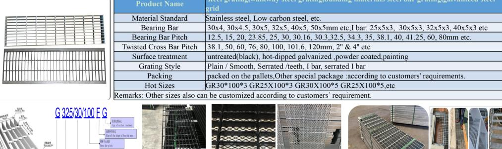
steel grating, walkway steel grating, building materials steel bar grating, galvanized steel
